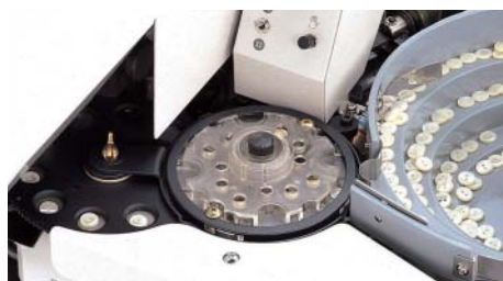
● Horizontal, forced feed mechanism
